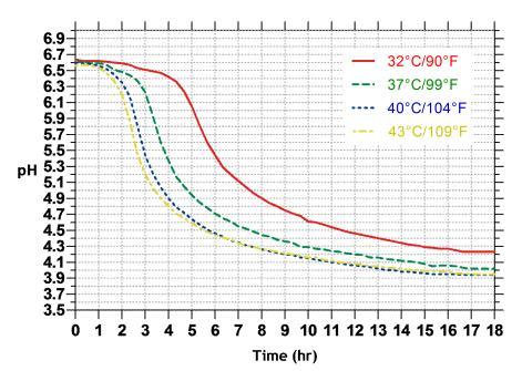
Fermentation conditions: Lab milk 9.5 % T.S.: 140°C/8 seconds - 100°C/30 minutes Inoculation: 500U/5000L
